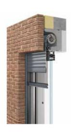
Above all, the system ensures free air circulation. The shutter box has a smaller size than the basic variant, which gives more possibilities for the external façade layer to be finished maintaining the same winding. Two revision options are available: from the inside or outside of the room, and the system can be fitted with an insect screen for extra protection against insects.
